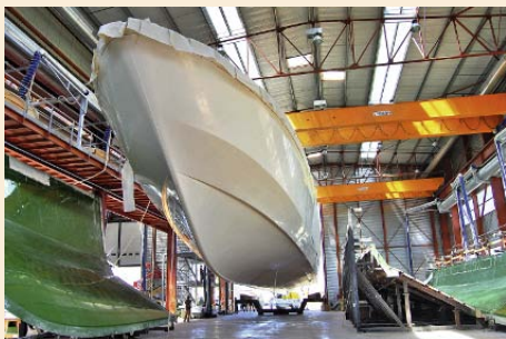
Couach 5000 Fly: The French yacht builders release the hull of the first 50-metre Couach from its mould.
